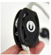
Step 4: Insert the small threaded screw into the plastic plate and tighten so that the screw passes through the rope and the end is slightly recessed from the edge of the trim block. The screw will thread between the fibers of the rope and will not jeopardize its strength.
